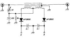
fig. 1. Schematic diagram of a conventional bridge arrangement for measuring SWR. The load across points A and B, if sufficiently low, will significantly affect the directivity as well as frequency response.
